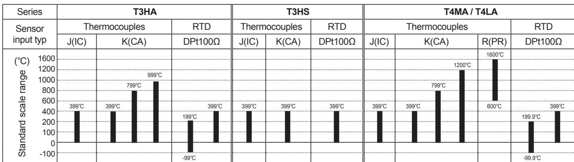
※ In case input sensor is R(PR) type, it is not available to perform correct control under 600°C.
