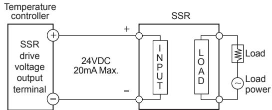
※When using voltage(for driving SSR) in the other purposes, do not over the range of the rated current.
