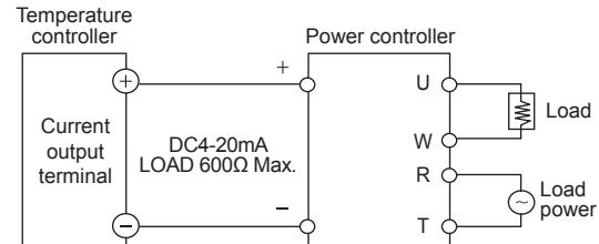
※The current value of DC4-20mA is available at lower than 600Ω of resistive load.
