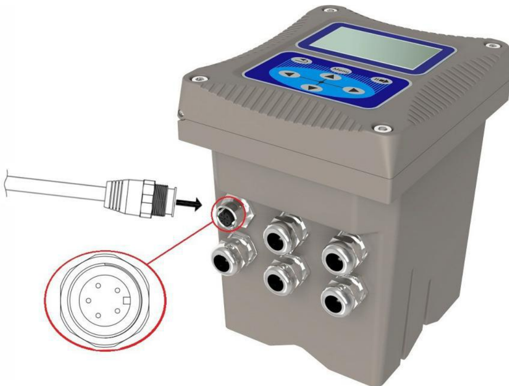
Figure 10 The Diagram of Sensor connection
