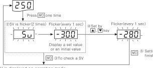
①PV is displayed on operation mode, ②Press MD key, the SV is indicated after "5" is flickering 2 times.
