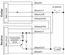
XIf the receiver OUT (black) line and the emitter JOB (black) line are not connected each other, the JOB indicator of the emitter is not operated and maintain the light status.
