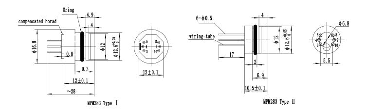
The suggested mounting dimension is  $\Phi12.6^{+0.12}_{+0.08}$ mm
