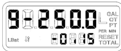
Figure 14: Linearisation point 9 (of 9)
