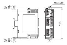
① Pull each Rail Lock switch up and down.
