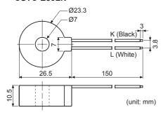
F=50Hz OUTPUT IN VOLTS RMS (V) Max. load current: 80A (50/60Hz) • Current ratio: 1/1000 • Wire wounded resistance: 31Ω±10% 0.001
