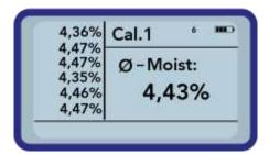
Within the operating mode "Average Value", the HD2 will deliver a representative measurement result of all measured locations that represents significant volume of the material.
