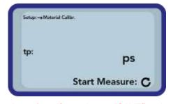
To start the measurement push the button "Measurement" . To increase the accuracy four measurements take place. The whole time of measurement is about 20 seconds. Afterwards the measured average impulse duration is shown for a short moment.
