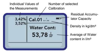
In order to delete the measurement series, actuate the button "Down"  $\blacksquare$ .
