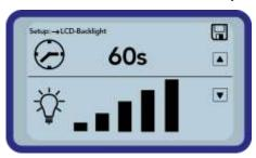
The selection of the background illumination, respectively the time until the automatic shut-down of the same is selected via the button "Up" by actuating the same several times. Using the button "Down" , you can adjust the intensity of the illumination, respectively turn the same completely off. Activate and store your settings by actuating the button "Measurement" . After activation, the symbol will appear in the upper right hand corner of the display.
