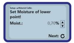
Next set the moisture oft the lower moisture point by pressing the buttons "Up" and "Down" .
