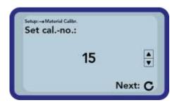
First you have to set the calibration curve to be changed (01 - 15)by pressing the buttons "Up" and "Down" .
