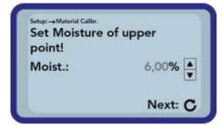
Next set the moisture oft the higher moisture point by pressing the buttons "Up" A and "Down" V.
