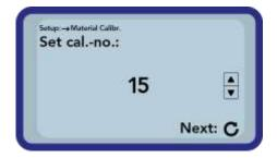
First you have to set the calibration curve to be changed (01 - 15) by pressing the buttons "Up"  $\triangle$  and "Down"  $\boxed{\square}$ .
