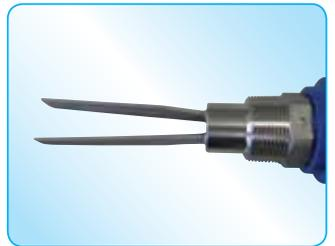
It shows the orientation of the vibrating forks after mounting. The mark have to be positioned face up, once installed on the side wall of the container. In case the orientation marking faces sideways, the working surface is too large:
