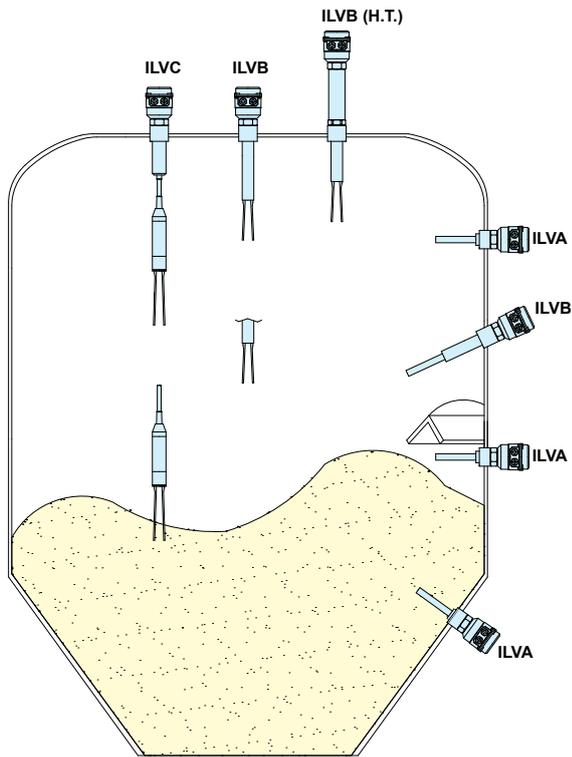
ILV Vibrating Level Indicators are fitted on the walls of a bin, silo or hopper, depending on the type of detection they have been installed for.
