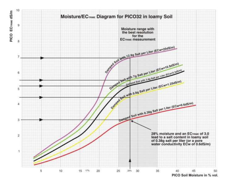
Also here the intersection point of "Moisture" and "EC<sub>TRIME</sub>" is representing the salinity curve EC<sub>w</sub> in the soil-diagram.
