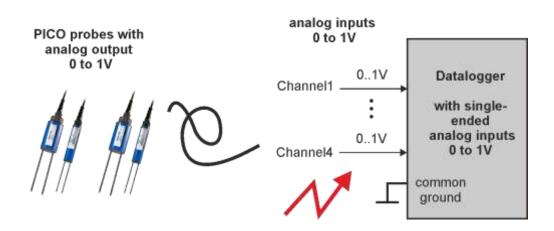
Recommends to use a datalogger with differential inputs as shown in the following picture. With differential inputs the problems with earth loops are eliminated.
