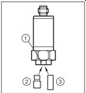
▶ Tighten the unit with a tightening torque of 8 Nm.
