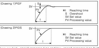
There are high-speed response type and low-speed response type built in this unit. Therefore user can select each function according to their application
