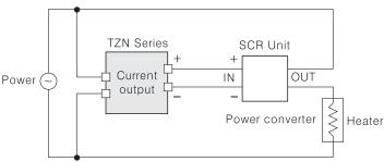
•It is important to select SCR unit after checking the capacity of the load
