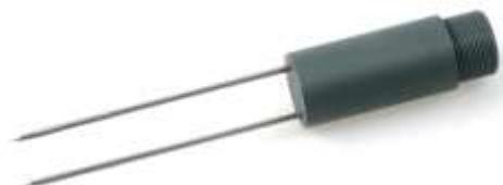
*For compacted, coarse or stony soil use the preparation set to bore a pilot hole!*
