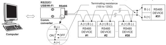
XIt is recommended to use Autonics communication converter; SCM-WF48 (Wi-Fi to RS485·USB wireless communication converter, sold separately), SCM-US48I (USB to RS485 converter, sold separately), SCM-38I (RS232C to RS485 converter, sold separately).
