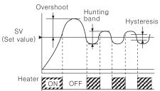
As like above picture, the control value is up and down by set value, it is called Hunting. And Overshoot is occurred at initial point when just power on. If the Hunting and Overshoot is less, it will be a good control.
