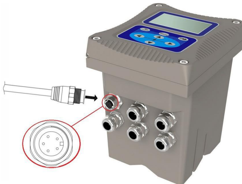
Figure 10 The Diagram of Sensor connection
