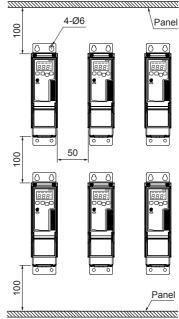
When installing multiple power controllers, please keep space at least 50mm in horizontal and 100mm in vertical between power controllers for heat radiation.
