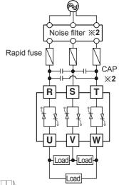
X1: This is only for models with RS485 communication output (SPR------). ※2: When connecting noise filter and capacitor, it is appropriate for EMC.
