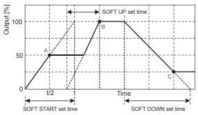
A: SOFT START function finished. B: SOFT UP function finished.
