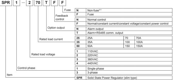
X1: Product is not equipped with a rapid fuse inside. Install the suitable fuse for rated load current of the model separately.
