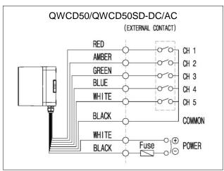
Power line and signal line are exposed to outside in case of LC type which is using external contact for sound tone selection.
