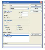
$OM_RS_Driver$  is used for controlling the RS485 communication, which is connected to input UN1.4 (L-, terminal 12) and UN1.4 (L+, terminal 12). A group of either inputs or outputs in the length of 1 Byte needs to be created in order to enter the parameters of this driver. The address of this Byte is not important, because  $OM_RS_Driver$  accesses the shared memory directly. Its setting can look like this example:
