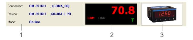
The information panel of the Device setup window contains basic data on <u>connection</u> (1), device display (2) and an image of connected device (3).
