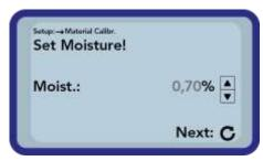
Next set the moisture oft the material by pressing the buttons "Up" and "Down" ...
