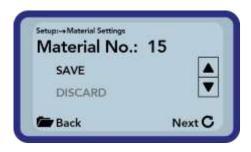
Finally you can store the calibration into the choosen calibration storage inside the probe. Choose "SAVE" an confirm by pressing the button "Measurement" C. If you choose "DISCARD" everything is left untouched.
