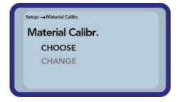
After the selection of the menu item "Material Calibration", you have to choose between "CHOOSE", to save one out of fifteen calibration as default calibration, or "CHANGE", to setup a new calibration in one of the fifteen calibration storages
