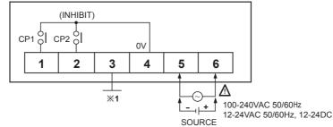
%1: It can be selected RESET or sensor power (+12VDC 50mA) by internal PIN operation. (Refer to J-40) ※CP1, CP2: Input signal terminals when using as counter.
