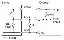
XPlease set R1 value to make the composed resistance of RL + R1 as Max. 470kΩ is an impedance for short-circuit. ※CP1, CP2 (INHIBIT), RESET input
