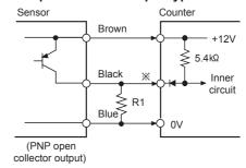
XIn case of PNP open collector output type sensor, please connect lower than 470Ω of R1 to input terminal before using.
