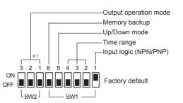
%1: Indicator model (FS5E-I4) does not have no. 1, 2, 3 of SW2 for output operation mode setting.
