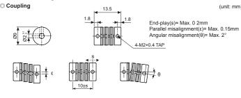
※Do not load overweight on the shaft. \*Do not put strong impact when insert a coupling into shaft. Failure to follow this instruction may result in product damage. %Fix the unit or a coupling by a wrench under 0.15 N m of torgue. When you install this unit, if eccentricity and deflection angle are larger. it may shorten the life cycle of this unit.
