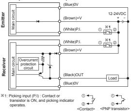
\*\*Picking indicator: When external picking input (P.I) is short-circuited with OUT (Black), it is operated same as ON/OFF status of control output.
