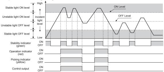
\*\*The above diagram is the state of operation for Light ON, but in case of Dark ON, it is opposite operation against Light ON.
