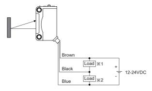
X1: Load connection of NPN open collector outputX2: Load connection of PNP open collector output
