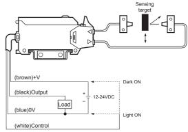
XEnables to use diffuse reflective type or through-beam type according to the fiber optic cable.
