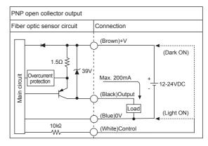
\*\*When selecting Dark ON or Light ON, please use control wire (White) Light ON: Connect control wire to 0V Dark ON: Connect control wire to +V
