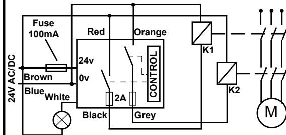
\*To protect safety line (internal 2A fuse), you can use external 1.6A fast fuse.
