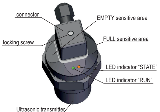
Key parts of the measuring device (version with Hall probes)
