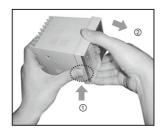
Pressing the front guide of Lock toward 1 and squeeze and pull toward 2, it is detached.
