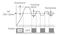
As like above picture, the control value is up and down by set value, it is called Hunting. And Overshoot is occurred at initial point when just
