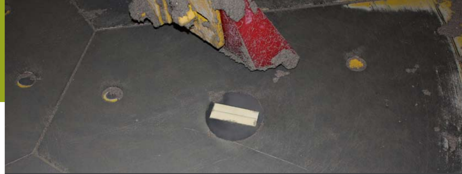
SONO-MIX moisture probe installed into a mixing pan bottom.
