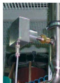
Monitoring of flow rates in pneumatic conveyor pipe with MicroFlow
