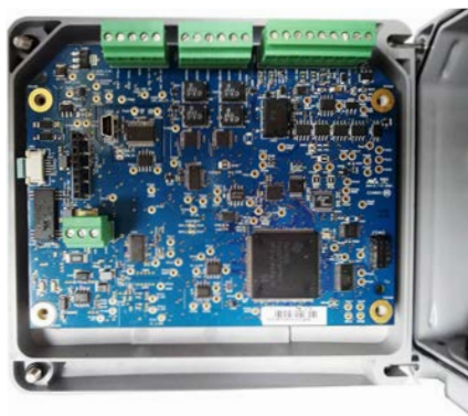
Figure 34: PCB shield removed
