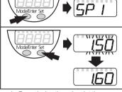
Numerical values are incremented continuously. For reducing the value: let the display move to the maximum setting value. Then the cycle starts again at the minimum setting value.
