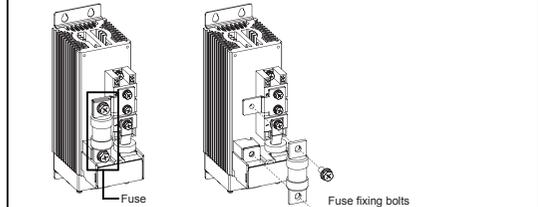
**Spec. of fuse fixing bolts**
