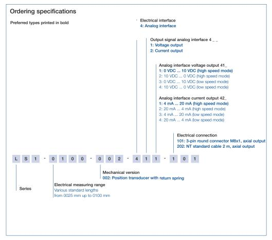
Output connector Cable Connector with cable Signal Code 202 EEM 33-56 /57 /-58 /-59 /-60 /-61 Code 101 Pin 1 GN green BN brown Supply voltage Pin 4 BK black WH white Output signal Pin 3 BN brown BU blue GND
