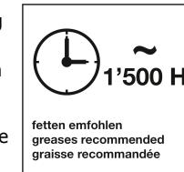
**NOTE:** Greases of different viscosity will reduce the operating frequency or can lead to the piston seizing as a result of the grease becoming resinous.
