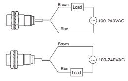
\*The load can be connected to either wire.
