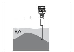
The system does not detect coverage by liquids similar to water.
