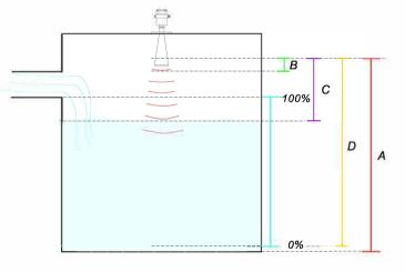
The unit measures the distance from the process connection of flange
