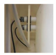
Capacitive proximity sensors belong to a sort of position sensors. Similar to the structure of a capacitor, the probe of sensor acts as one pole of capacitor and another pole is the sensing object. While the sensing object approaches a proximity sensor, the dielectric constant may change between object and sensor. Meanwhile, this causes the circuit to alter.
